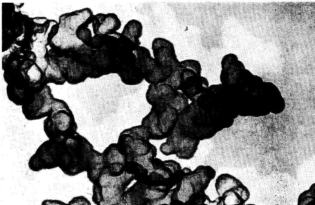
FIG. 2. Electron micrograph of platinum shadowed carbon replica of palladium black B ( \times 113,000 ).
