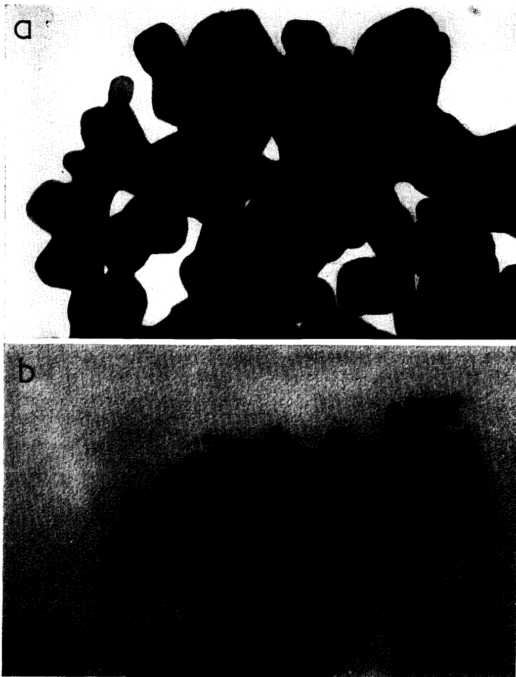
FIG. 1. Direct transmission electron micrographs of: (a) palladium black A ( \times 272,000 ); and (b) palladium black E ( \times 482,000 ).
